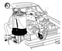
Mount the oil suction hose on Open the valve on the oil suction pipe and complete the oil suction process (HU 0159).
